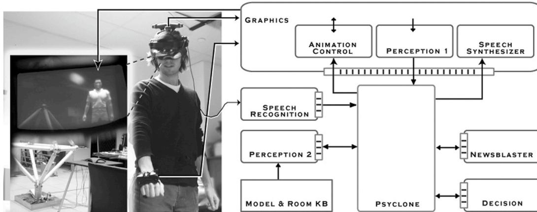
**Figure 2. Mirage system architecture, showing sensor and display connections to the physical devices. Arrows to and from Psyclone indicate message and control flow. Small striped rectangles on the edges of modules signify Psyclone adapters.**
